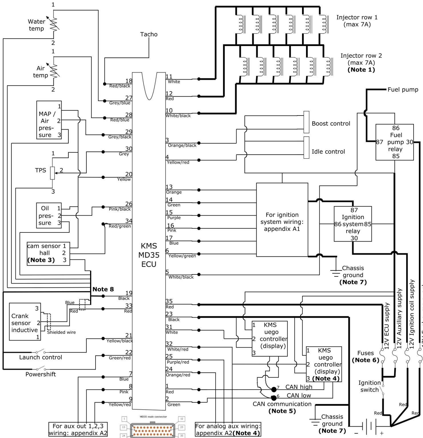
**Note 1:** A maximum of 6 high impedance injectors can be used on one injector output. When using low impedance injectors or more than 6 high impedance injectors on one injector output, an external KMS injection driver (2x10A) needs to be used. For connection of the injection driver, see wiring examples.
